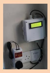
Bytronics Web Weight Indicator module is a hardware interface module that allows any web application to receive weight data from any digital weight indicator with rs232 communication support. The module has a configuration for setting up a web page that receives the weight data.
