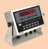
The 420 Plus is a single-channel digital weight indicator housed in a NEMA Type 4X/IP66-rated stainless steel enclosure. The indicator front panel consists of a large (.8 in, 20 mm), six-digit, and seven-segment LED display and twenty-one-button keypad. Features include:
